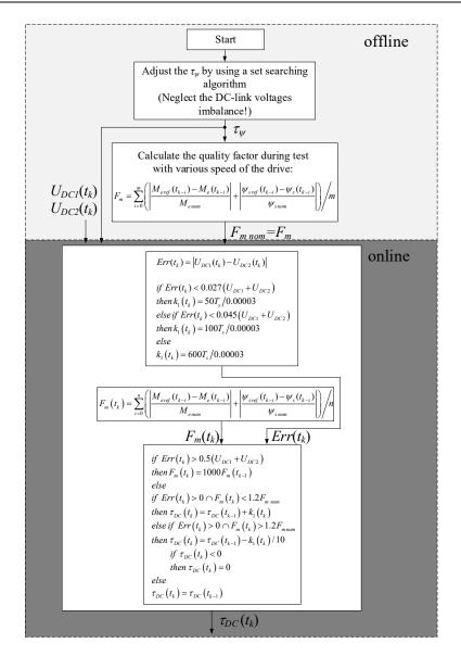
Fig. 2. Fitting procedure of weighting factors
