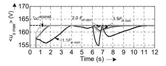
Fig. 7. Mean value of maximal inverter voltage  $u_{s \max}$  that can be generated in linear modulation mode of the inverter for various control quality requirements
