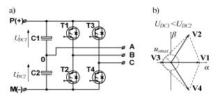
Fig. 1. Four-switch inverter topology (a) and a maximal voltage vector  $u_{s \max}$  under DC-link voltage imbalance (b)
